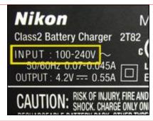
Most electronic devices have a prominent label that looks like this picture. On this device (a camera battery charger), you can see that after "Input" it says "110 – 240V", which means that it can be used with any voltage within that range, including the 110V standard in Canada or the 220-230V standard in much of Europe. All you will need is a plug adaptor.
