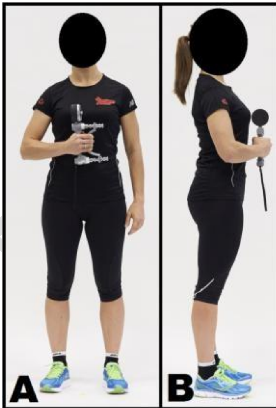
Figure 3.1: Frontal (A) and Sagittal (B) View of the Correct JAMAR® and Body Position to Conduct the Relative Handgrip component
